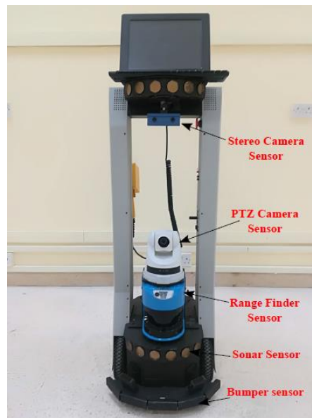
Figure 2. The PeopleBot mobile robot platform, where several sensors are attached to the robot (e.g. pan-tilt-zoom (PTZ) camera, laser range finder, sonars, stereo camera, ...etc.).
