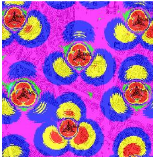
Figure 4. Signal strength from empirical propagation predictions [31].
