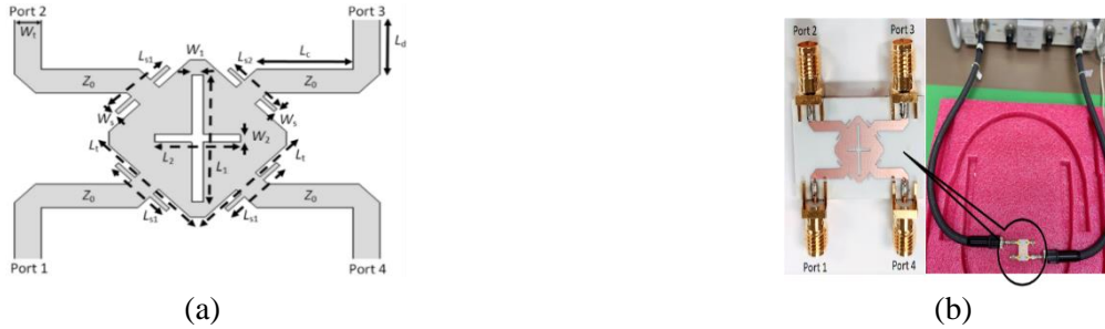
Figure 4. 3 dB/90° patch coupler with loaded stubs (Design B): (a) Physical topology; (b) Photograph under test.
