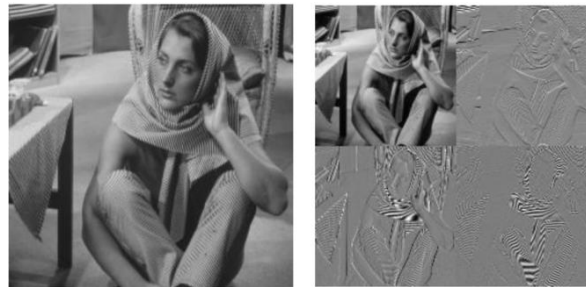
Figure 2. The original image to the left and its DWT to the right.
