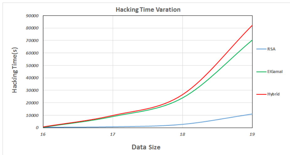
Figure 3. Comparison of performance and efficiency of the classical RSA and ElGamal cryptosystems with the innovative combined RSA-ElGamal cryptosystem across data sizes ranging from 10^{16} to 10^{19} (approximately 54 to 64 bits).
