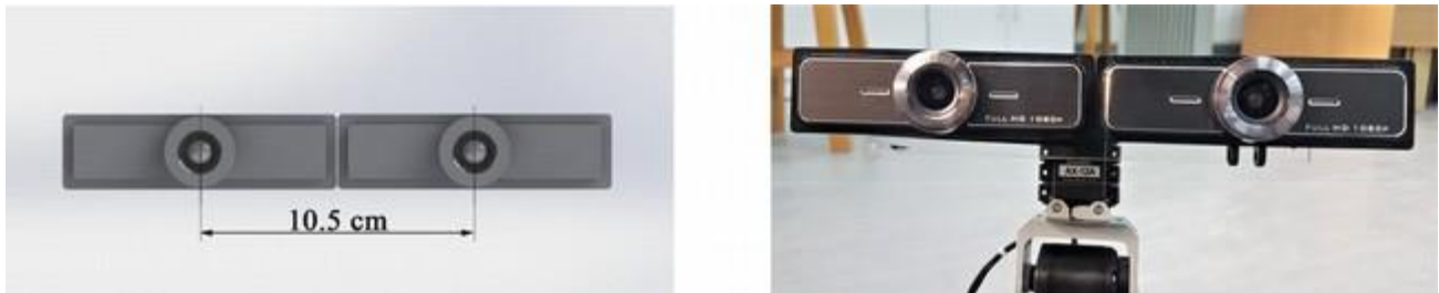
(a) Stereoscopic camera model, (b) Actual developed design of the stereoscopic camera set
