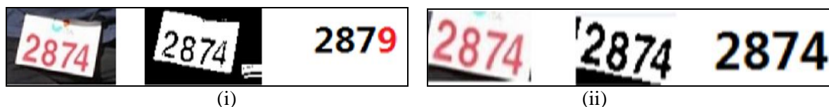
Figure 2. Binarization and recognition results for input images (i) without torso detection (ii) with torso detection [3].
