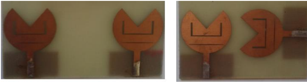
Figure 5. Pictures of the fabricated MIMO configurations.
