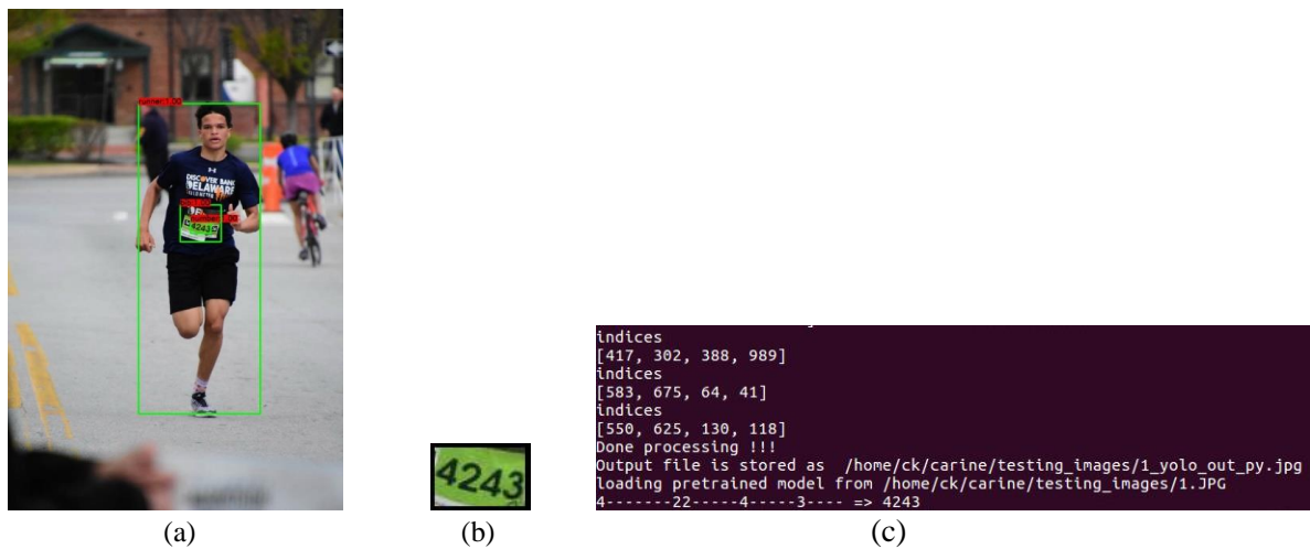
Figure 11. Demonstration of RBN detection and recognition cascade network: (a) Objects detected using YOLOv3 model, (b) Bounding box of RBN cropped image (c) Recognition process using CRNN model.
