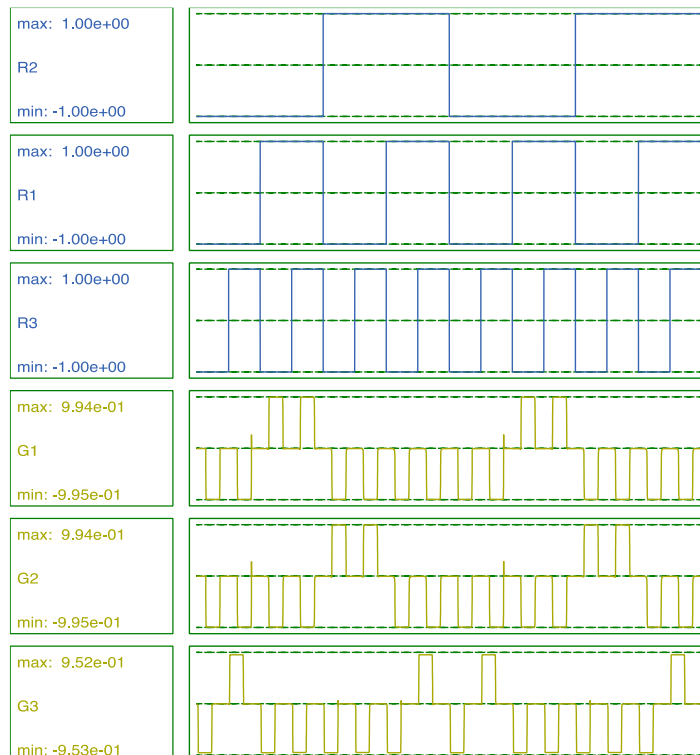
Figure 13. Simulation results of 3-input arbiters - Design B.
