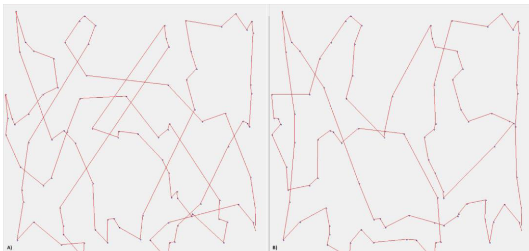
Figure 8. The resultant routes after applying the GA and CSGA methods on kroA100 instance; (a) GA, (b) CSGA.
