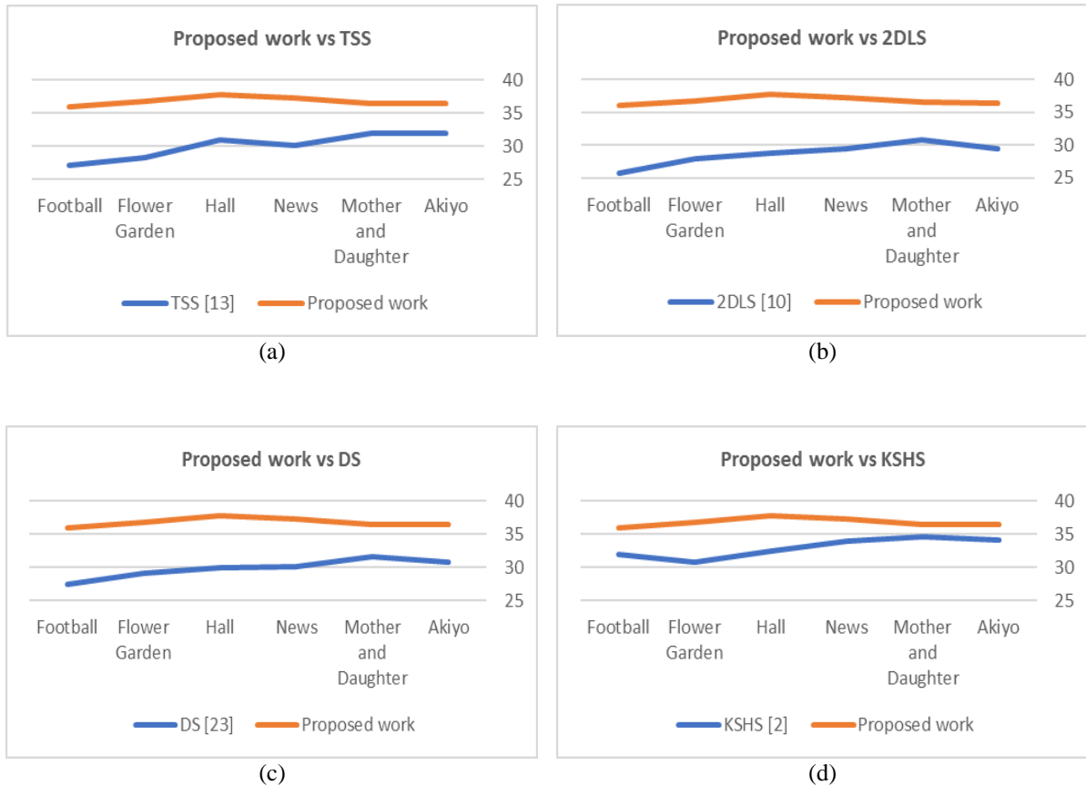
Figure 3. Visual representation that compares the proposed work with well-known algorithms as follows: (a) three-step search, (b) two-dimensional logarithmic search, (c) diamond search, (d) Kalman simplified hierarchical search.
